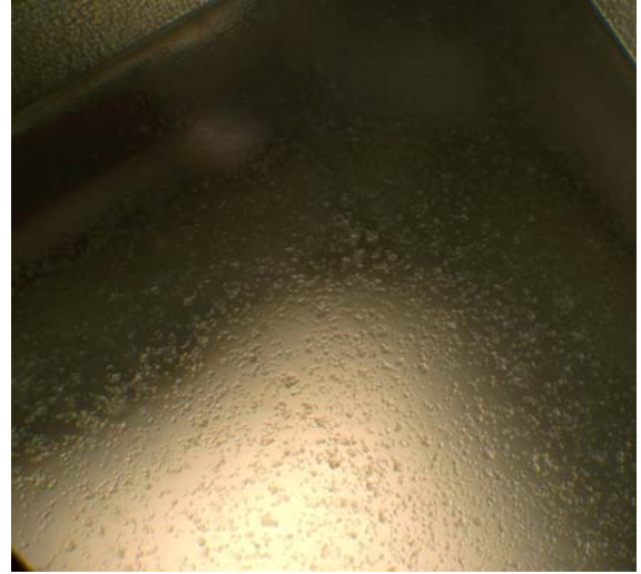
B) After 1 Cycle of 1 Minute Positive Corona Followed by 1 Minute Negative Corona
