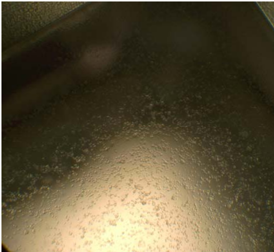
C) After 2 Cycles of 1 Minute Positive Corona Followed by 1 Minute Negative Corona
